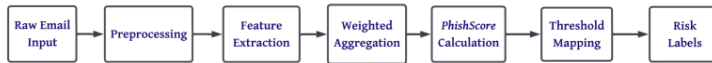
Figure 3.1: PhishScore system architecture: a six-stage pipeline from raw email input to risk-level output.
