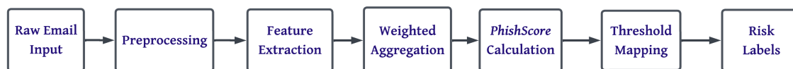
Figure 3.1: PhishScore system architecture: a six-stage pipeline from raw email input to risk-level output.
