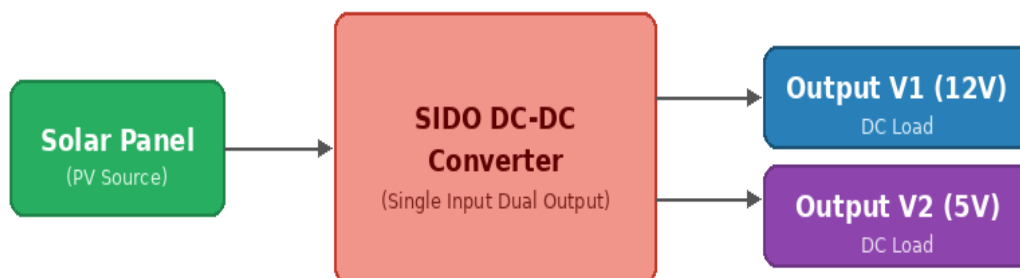
Fig 4.1.1 Block diagram of Solar Panel
