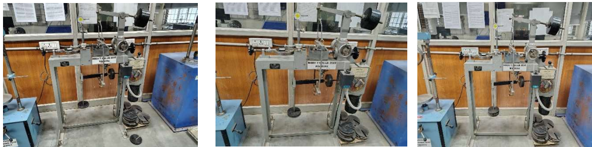
Fig. 3.7 Experimental setup of DST subjected to a normal stress of 0.5, 1 and 1.5 kg/cm 2 (Soil Mechanics Laboratory, DTU, Delhi)
