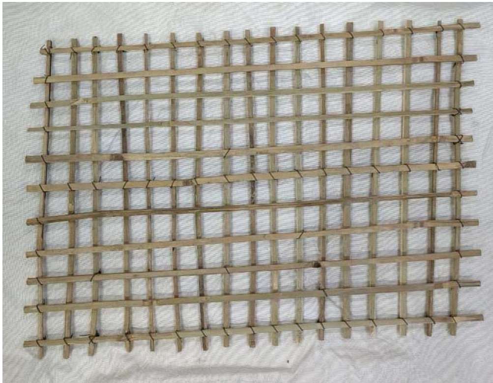
Fig. 3.14 Bamboo grid used for reinforcement
