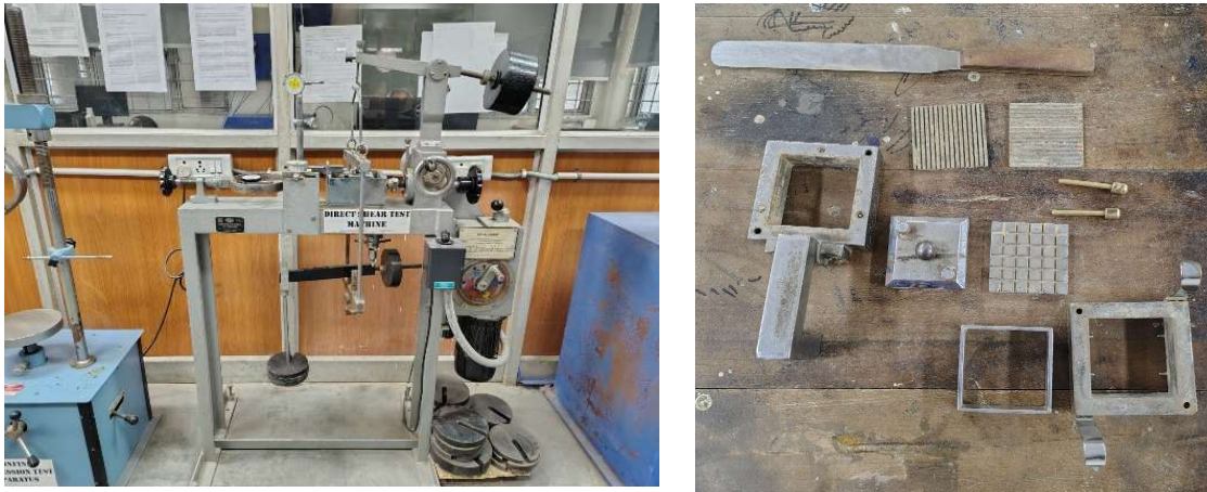
Fig. 3.6 Direct shear testing system consisting of test setup
