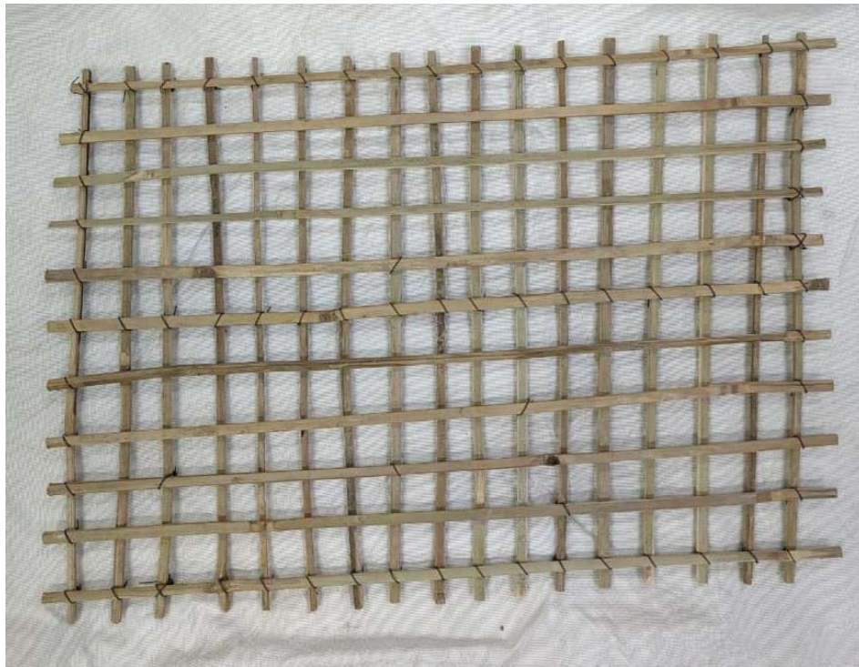
Fig. 3.14 Bamboo grid used for reinforcement
