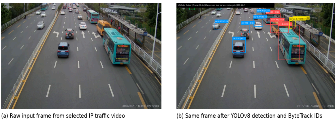
Figure 3.2: YOLOv8 input frame and corresponding detection output from the selected traffic video.
