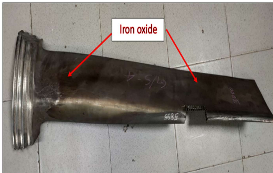
Figure 3.2: Black patches (Iron Oxide ( \text{Fe}_3\text{O}_4 )) observed on the blade's surface
