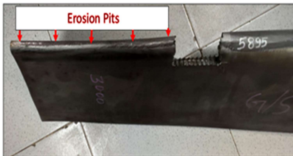
Figure 3.3: Erosion pits at the blade aerofoil-leading edge.
