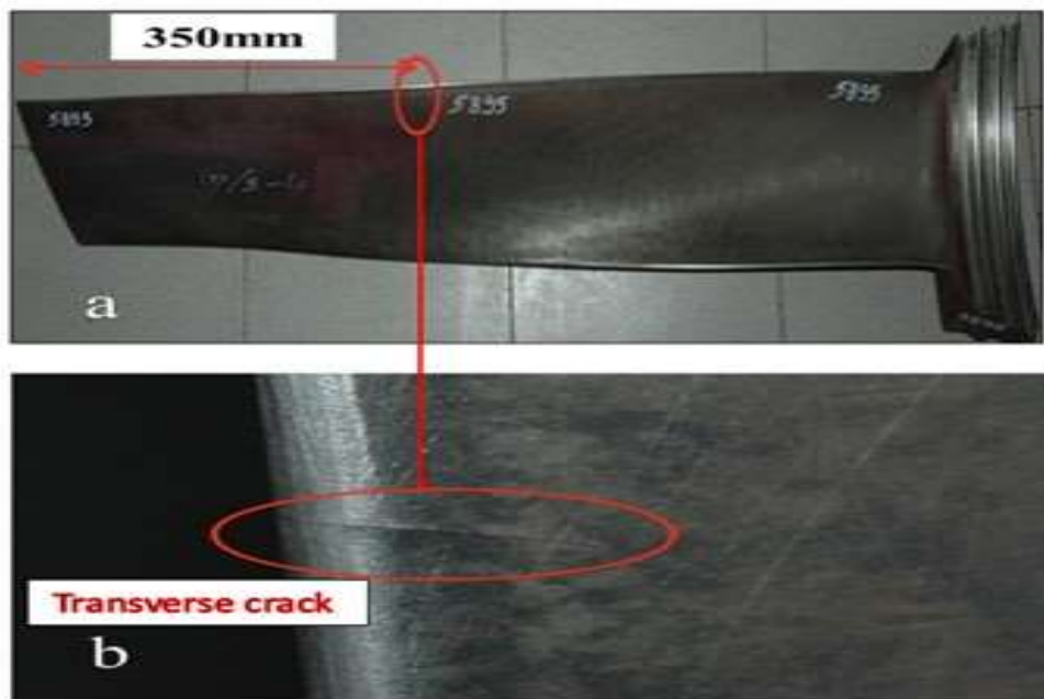
Figure 6.1: (a) Location of crack (b) Transverse crack on the leading edge of L-0 LPST blade
