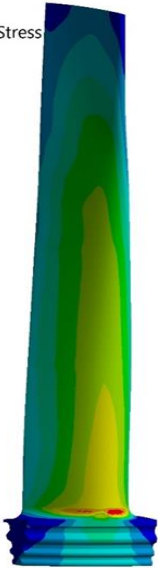
Figure 6.6: Equivalent stress of LPST blade
