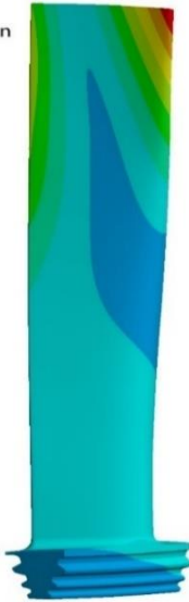
Figure 6.7: Total Deformation of LPST blade
