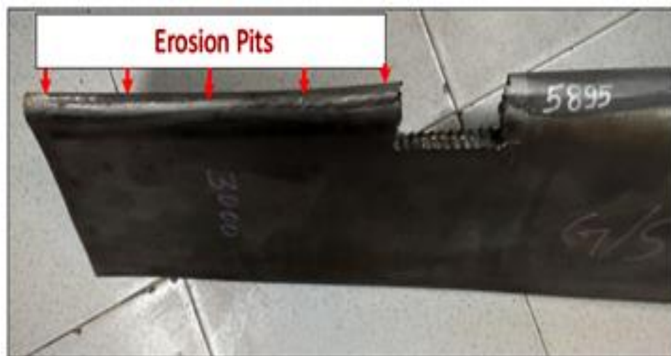
Figure 3.3: Erosion pits at the blade aerofoil-leading edge.
