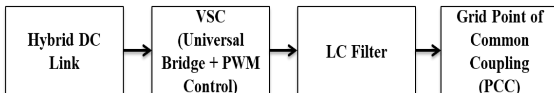
Fig 2.1 Functional block diagram of the VSC showing the DC-link interface, control system, and grid connection.
