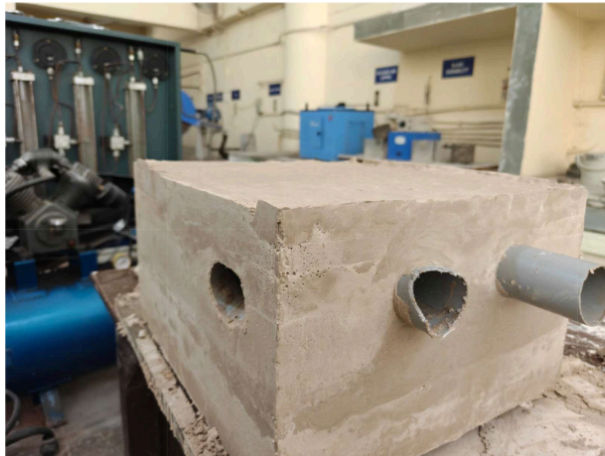
Fig 8. Tunnel model casted in Plaster of Paris
