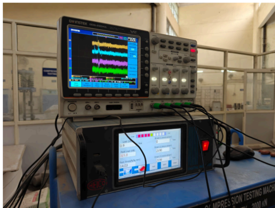
Fig 12. Data acquisition from 4 channels through PZT sensor in Oscilloscope
