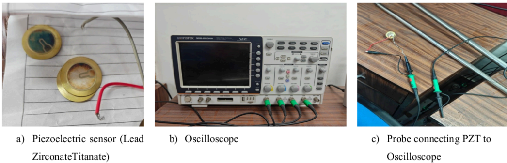
Fig 9. Instruments used in Monitoring of tunnel behaviour
