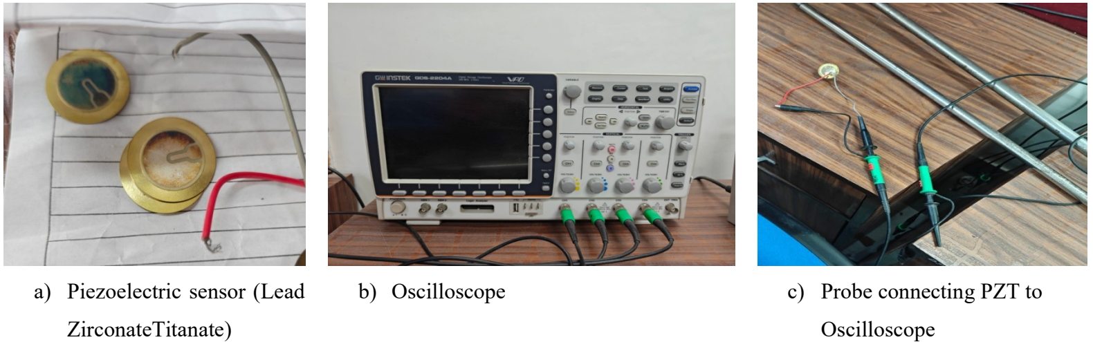
Fig 9. Instruments used in Monitoring of tunnel behaviour
