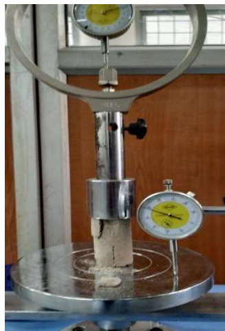
Figure 6.8: sample prepared for UCS test with the help of sampler, Figure 6.9: Loading cell with failed sample, Figure 6.10: failed sample.
