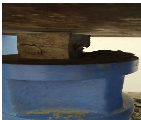
Figure 3.5: a) Failed sample in CTM loading
