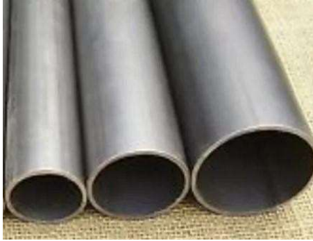
Figure 3.3. Pipes used for making stone column
