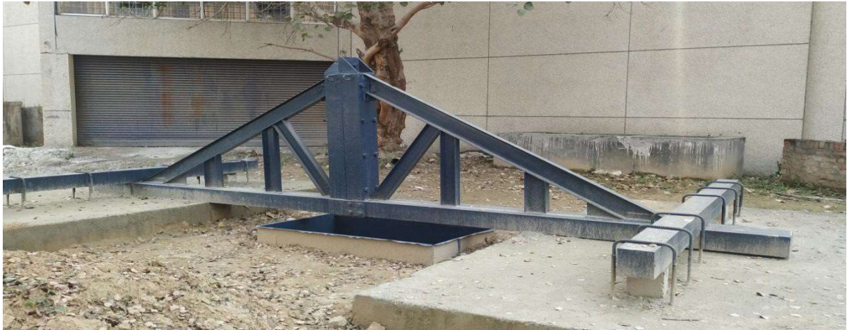
Fig 3.1: Model Test Tank with Loading Frame
