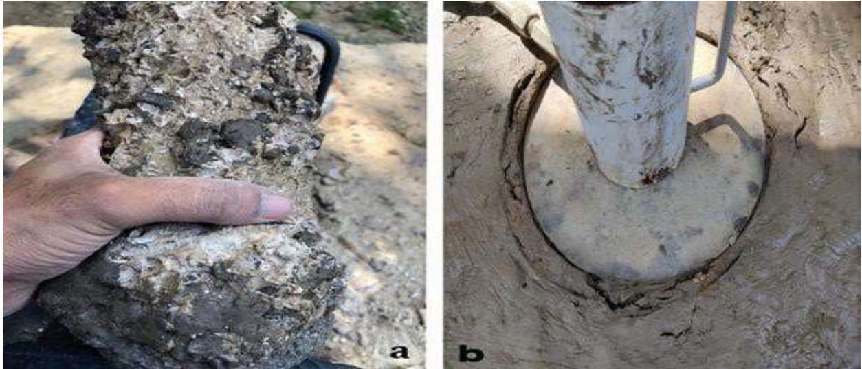
Figure 4.17 (a) Bulb is developed at the base of the column due to punching failure; (b) cracks developed at the surface due to punching.
