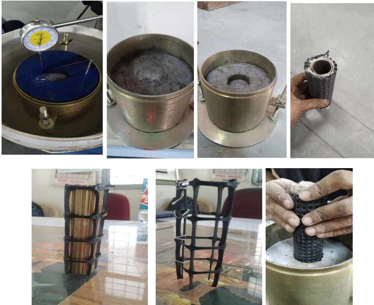
Figure 6.1: sample soaked in water for 96 hours, Figure 6.2: sample after soaking for 96 hours with single end bearing column, Figure 6.3: failed sample after loading with single column, Figure 6.4: column casing with encasement using geotextile, Figure 6.5 & Figure 6.6: column casing with geogrid, Figure 6.7: placing of encasement with casing in expansive soil.
