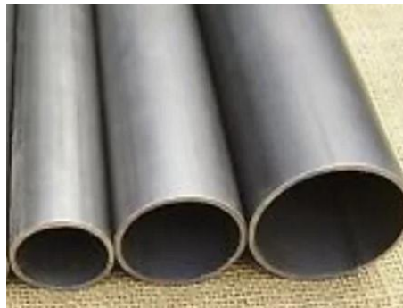
Figure 3.3. Pipes used for making stone column
