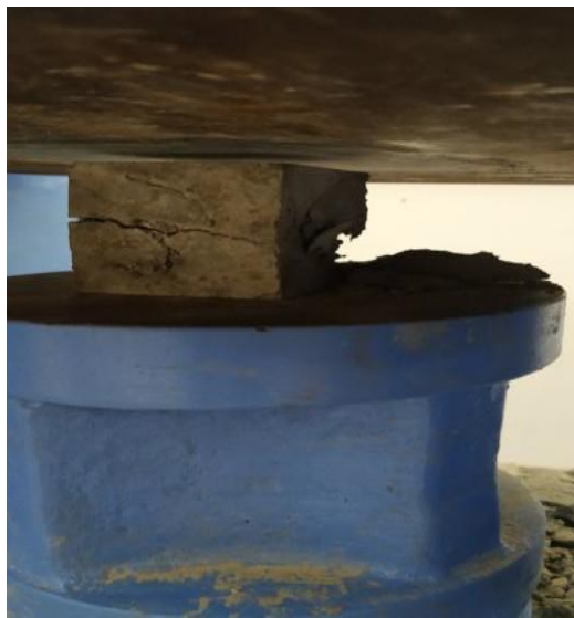
Figure 3.5: a) Failed sample in CTM loading
