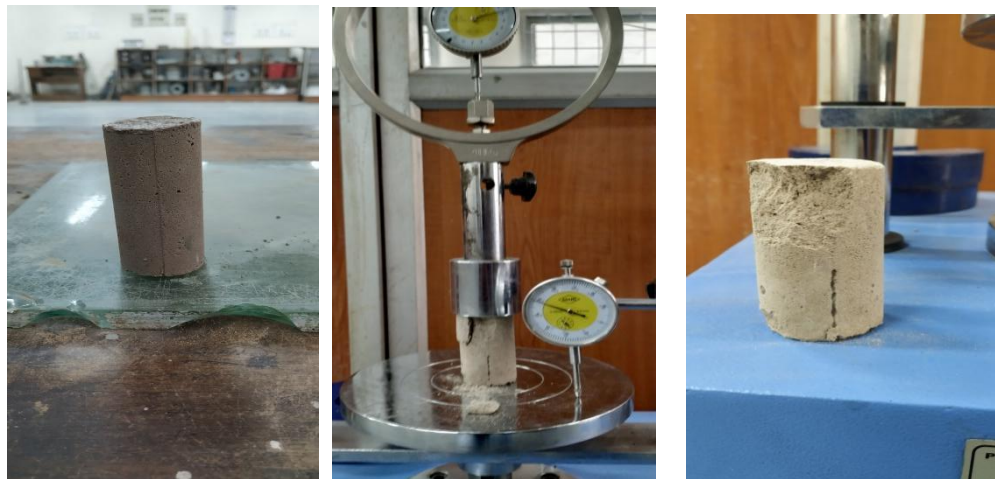
Figure 6.8: sample prepared for UCS test with the help of sampler, Figure 6.9: Loading cell with failed sample, Figure 6.10: failed sample.
