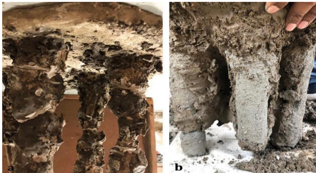
Figure. 4.18: (a) Exhumed square pattern column; (b) exhumed hexagonal column.
