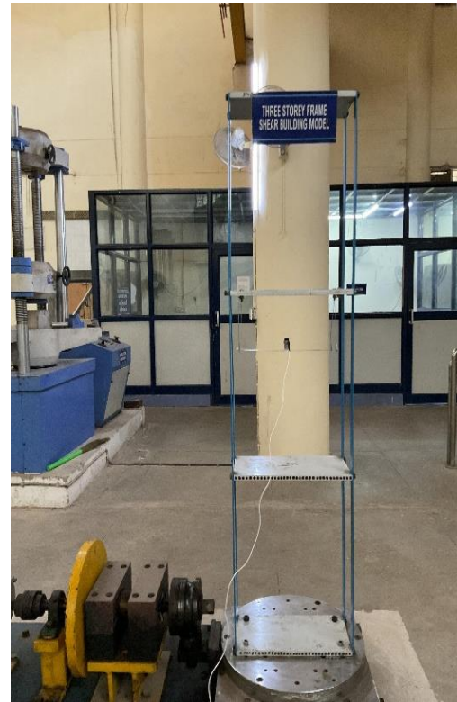
b) Cable tray attached at 2 nd floor slab
