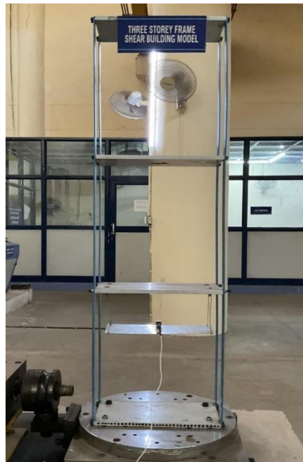
Figure 3.2 Three storey frame model
