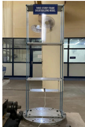
Figure 3.3 Three storey frame model
