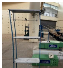
c) Accelerometer attached at centre of the cable tray
