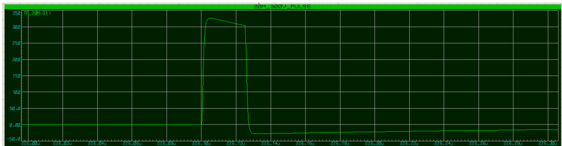
Figure 3.5: 20MHz 300V Output Pulse)
