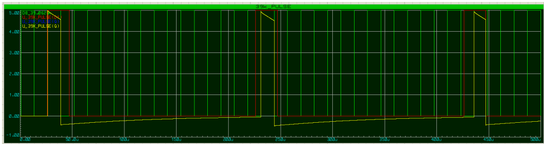
Figure 3.17: 625kHz pulse logic a) 39.0625kHz input pulse(Green) b)Repetition control signal(Red) c) Isolated 39.0625kHz pulse(Yellow)
