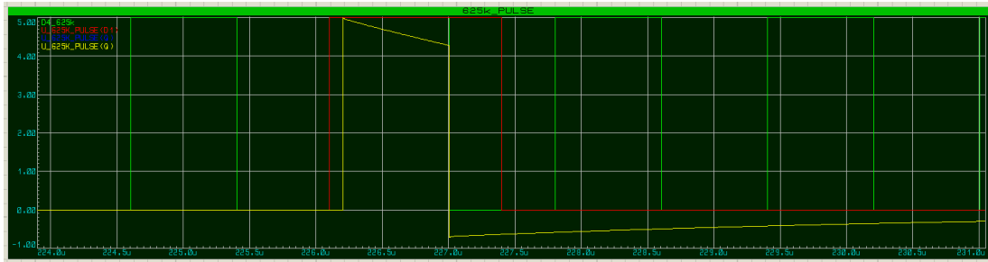
Figure 3.10: 625kHz pulse logic a) 625kHz input pulse(Green) b)Repetition control signal(Red) c) Isolated 625kHz pulse(Yellow)
