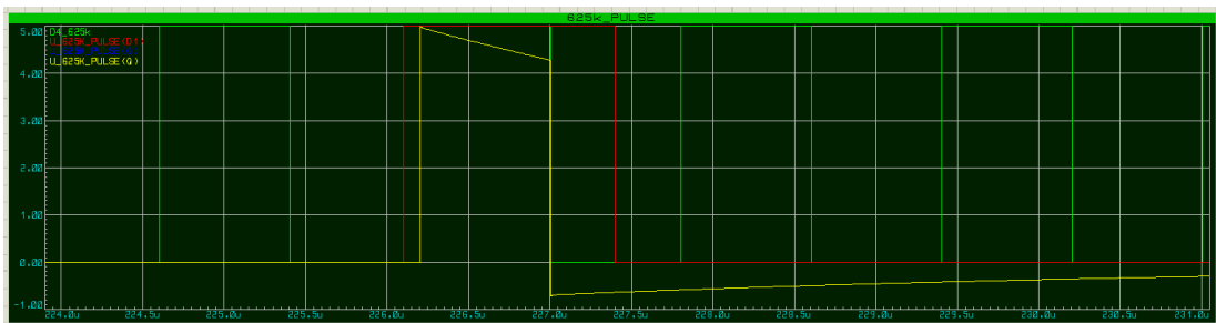
Figure 3.10: 625kHz pulse logic a) 625kHz input pulse(Green) b)Repetition control signal(Red) c) Isolated 625kHz pulse(Yellow)
