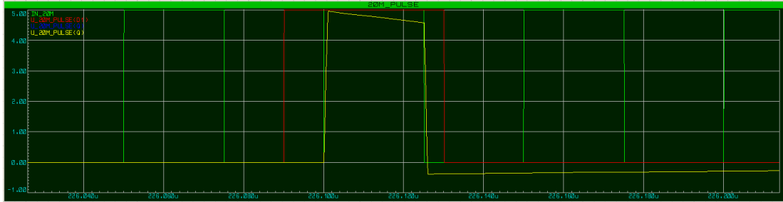
Figure 3.4: 20MHz pulse logic a) 20MHz input pulse(Green) b)Repetition control signal(Red) c) Isolated 20 MHz pulse(Violet)
