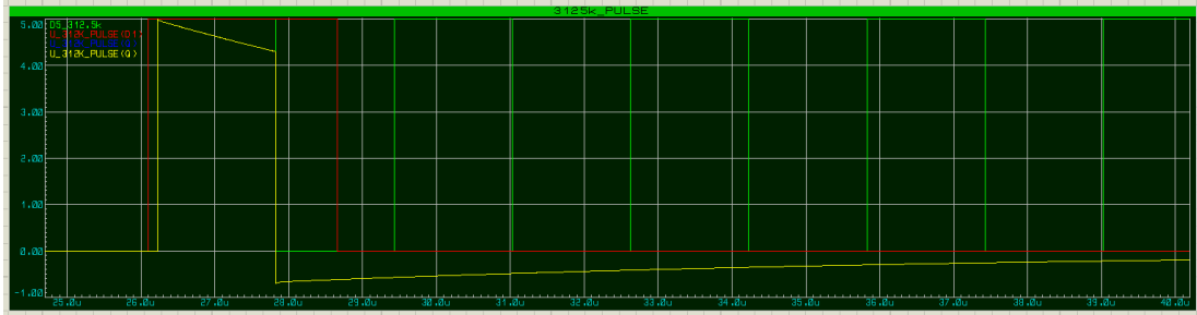
Figure 3.13: 312.5kHz pulse logic a) 312.5kHz input pulse(Green) b) Repetition control signal(Red) c) Isolated 312.5kHz pulse(Yellow)
