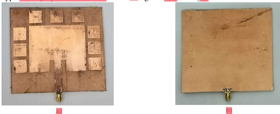
Fig. 3. The proposed prototype of an implanted antenna: (a) top view, (b) back view
