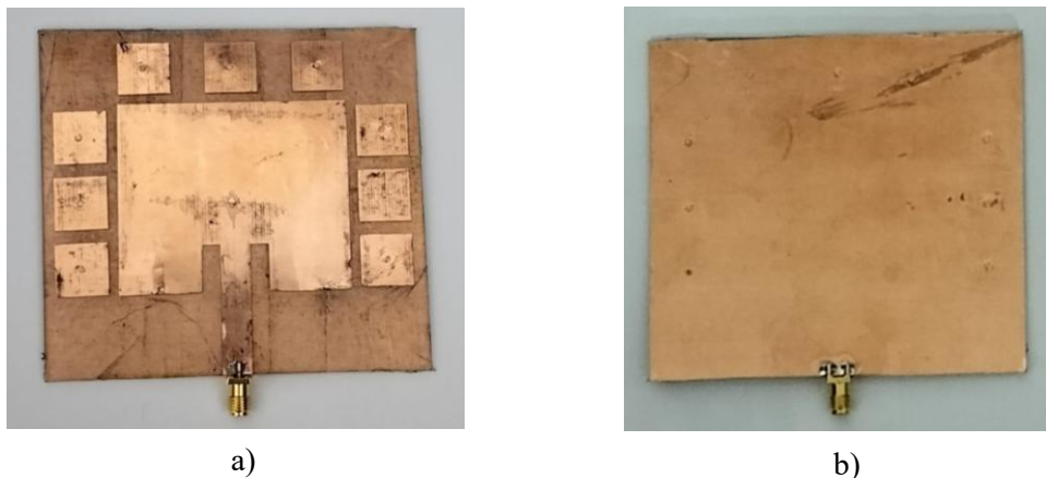
Fig. 3. The proposed prototype of implanted antenna: (a) top view, (b) back view
