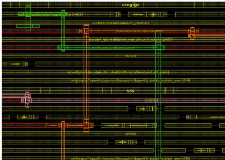
Fig. 6.6: Dummy fills overlapping on signal nets
