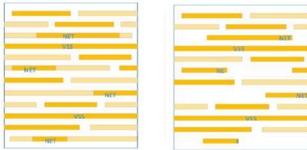
Fig. 5.2 Dummy fills and signal nets (a) signal nets overlapping on dummy fills. (b) Intersecting dummy fills are removed leaving only signal nets. [11]
