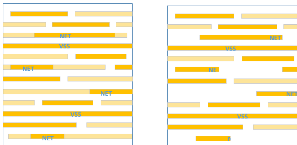
Fig. 5.2 Dummy fills and signal nets
