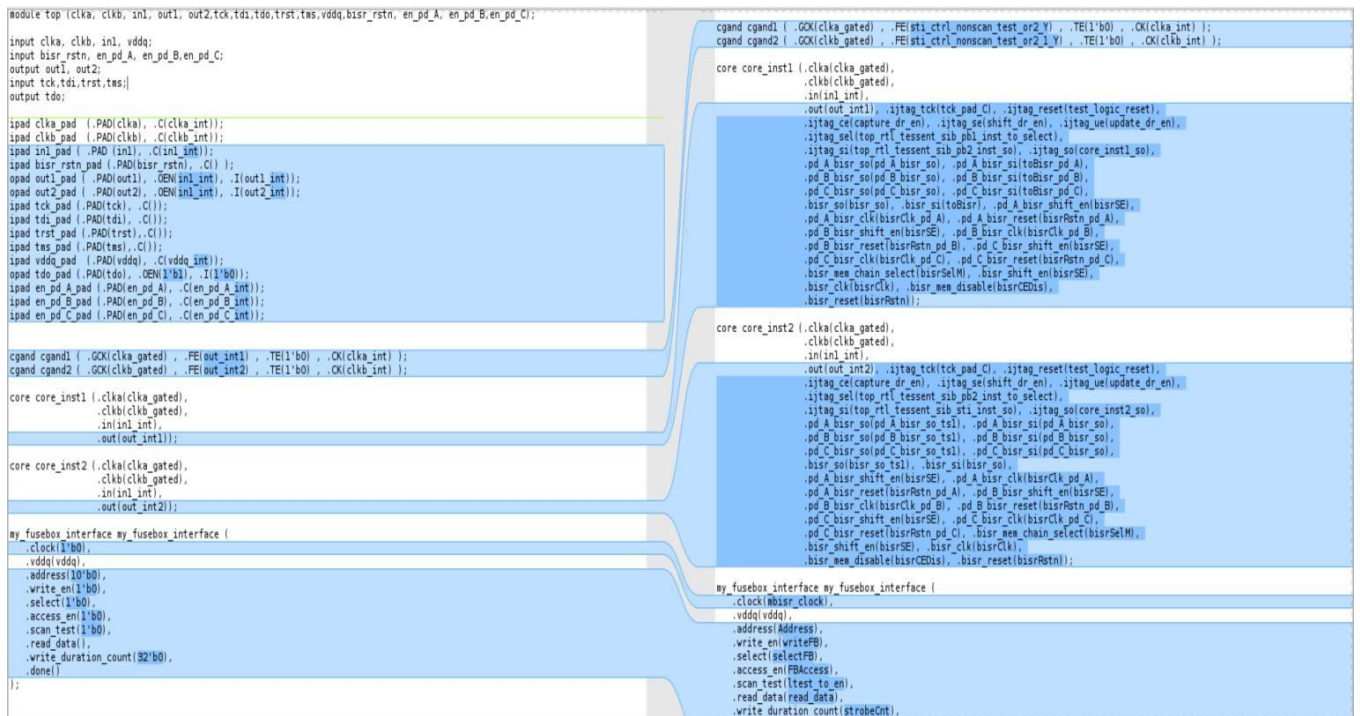
Figure. 4.4 Additional instances that got added post MBIST insertion
