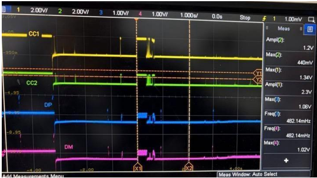
Figure 4.37: CC Pin OverVoltage Protection Response of Injonic IC
