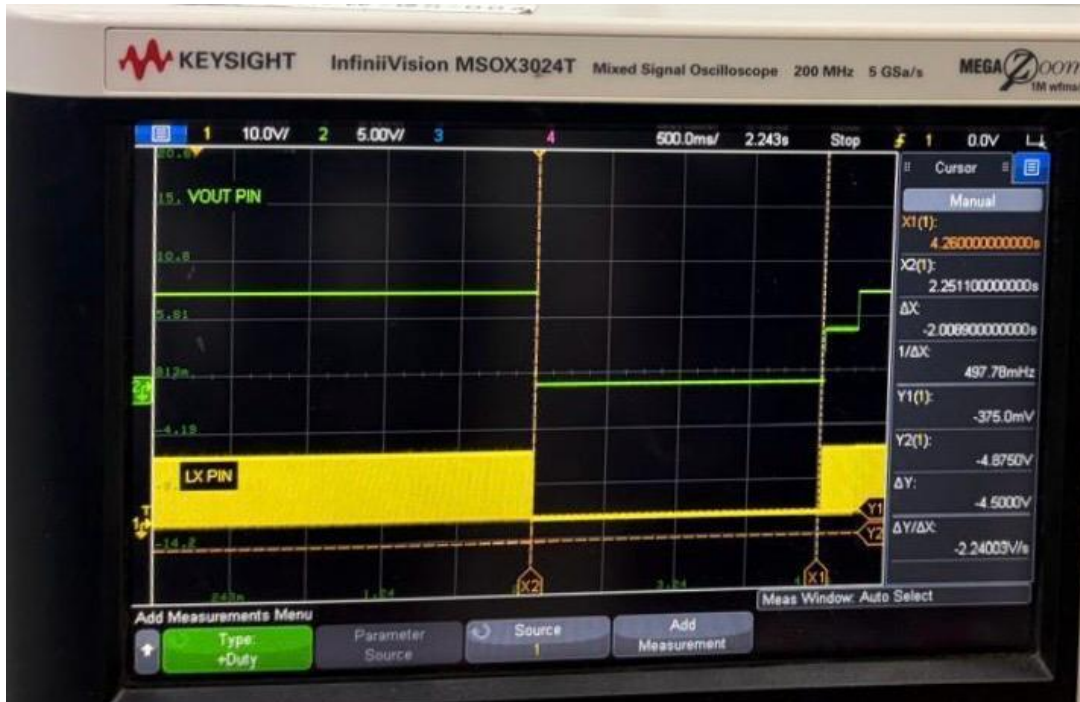
Figure 4.33: SC Protection Response of Injoinic IC Observed on Oscilloscope
