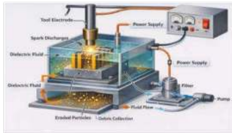
Figure 1.18 Electro-Discharge Micromachining process [88]
