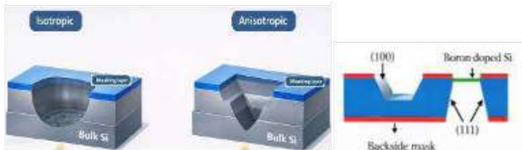
Figure 1.14 Bulk Micromachining process [83]
