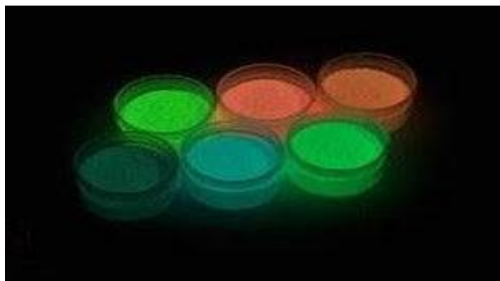
Figure 1.3: Photoluminescent Material (glow in dark)
