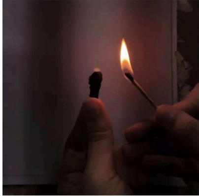
Figure 7 The developed peel- based bioplastic exhibited high heat resistance converting into ash rather than melting when exposed to flame, confirming its non-thermoplastic and biodegradable in nature
