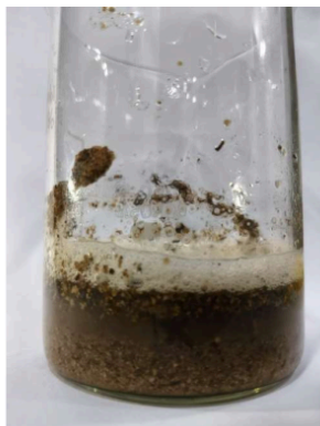
Figure 3 Submerged the sample into the distilled water and heated upto approximately 100°C to soften the peel tissues.
