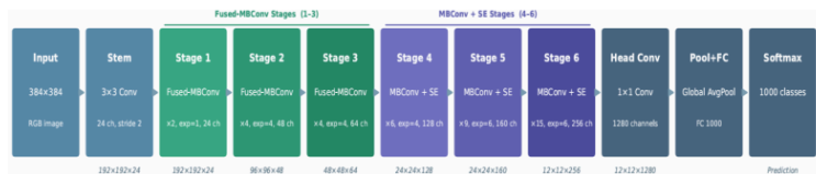
Fig. 4: Architecture of EfficientNetV2-S (Classes are 1000 as it is trained on ImageNet dataset, after fine-tuning to current dataset 5 classes are there)
