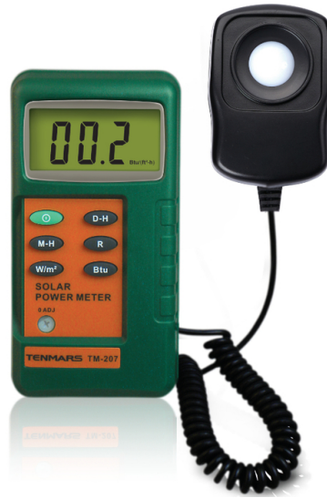
Figure 4.2: Tenmars TM-207 Solar Power Meter
