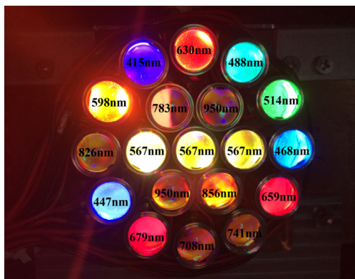
(a) LED arrangement with different peak wavelength
