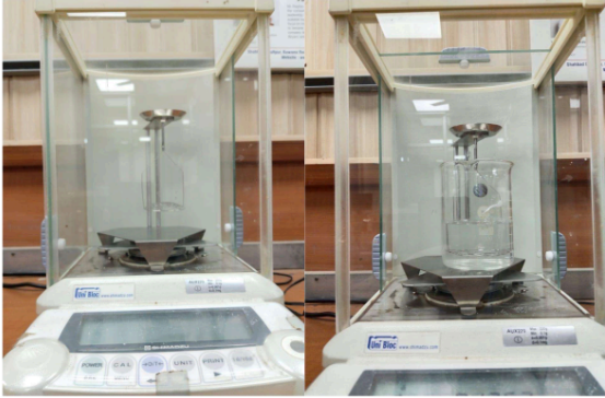
Fig 3.5: Porosity measuring apparatus
