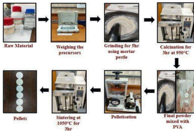
Fig. 2.1: Pictorial representation of synthesis of BaBi 2 Nb 2 O 9 (BBN) ceramics doped with Nd 3+ ions.
