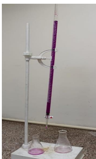
Fig 3.3: Experimental Setup used for KMNO 4 titration analysis
