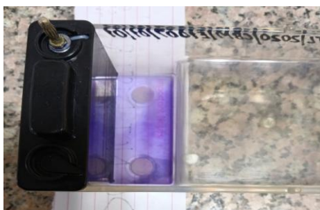
Fig 4.5: Crystal violet retention observed in the electrophoretic chamber after 72h incubation.
