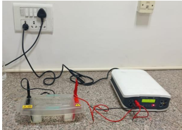
Fig 3.2: Electrophoretic chamber connected to DC power supply used for electric field-assisted microbial treatment.
