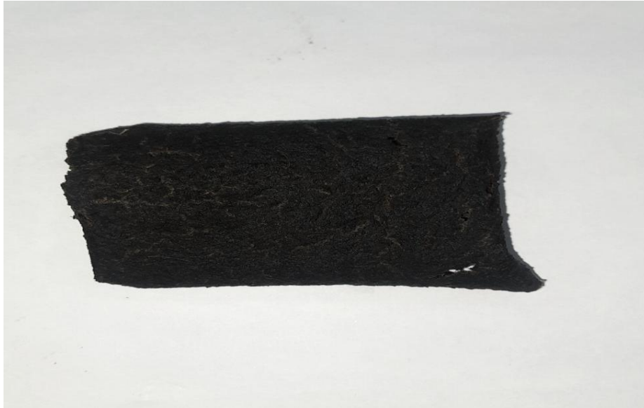
Figure 4.1 Bioplastic synthesised from powder of Green banana peels and Potato Peel
