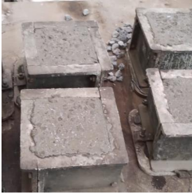
Figure: 6 Concrete moulds filled with fresh concrete
