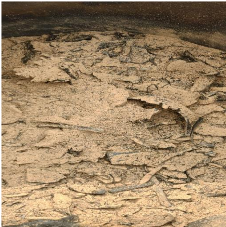
FIG: 1 COCONUT SHELL ASH
