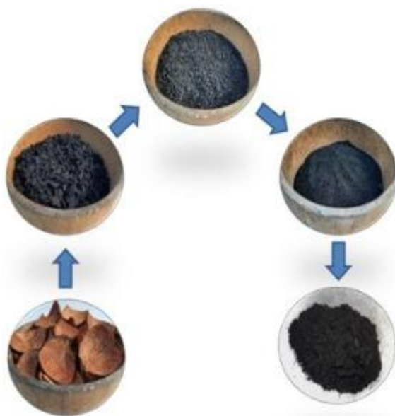
FIG 3: FORMATION OF COCNUT SHELL ASH
