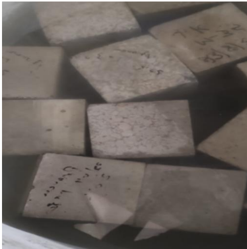
Figure: 8 Concrete cubes in a concrete water tank
