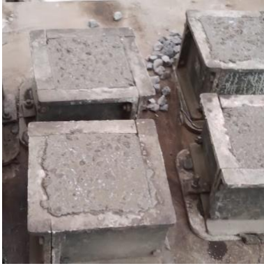
Figure: 6 Concrete moulds filled with fresh concrete
