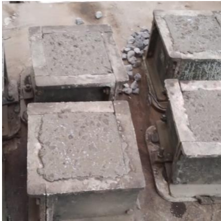
FIGURE: 3 CONCRETE MOULD OF CONCRETE
