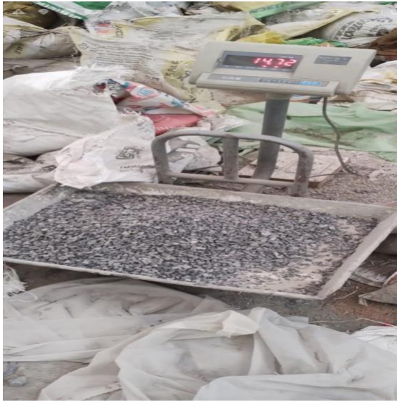
FIGURE: 5 WEIGHT OF AGGREGATE
