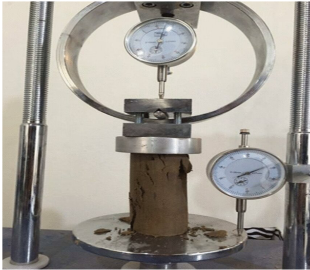
Fig. I.4 : Unconfined compressive strength test on soil sample
