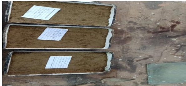
Fig 13: compacted bed after spraying solution
