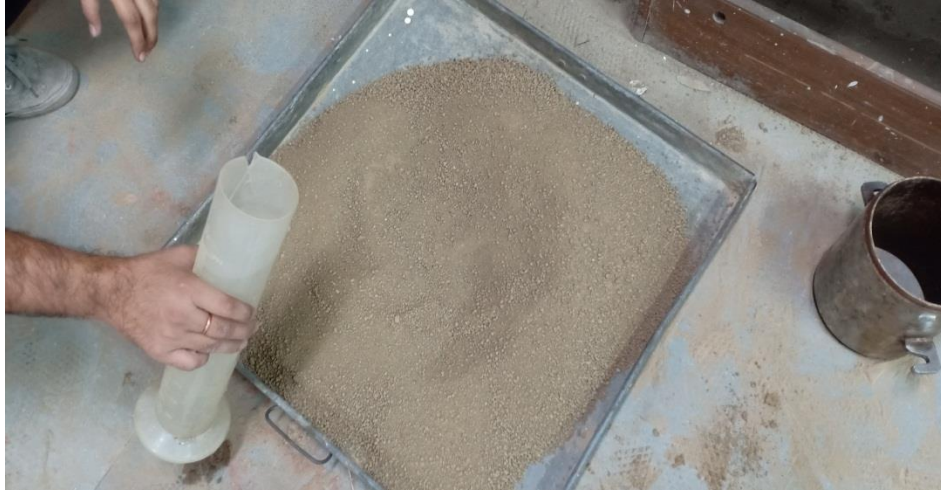
Fig 9: Mixing OMC in dried soil sample
