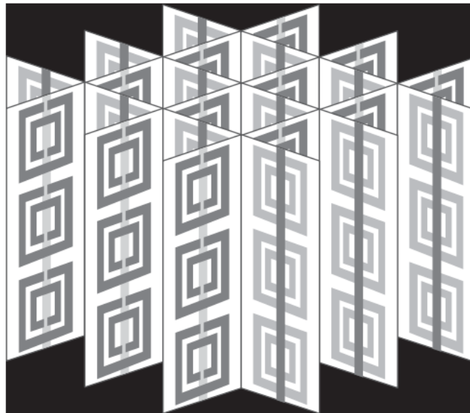
Fig. 2.5: Array of Split Ring Resonators with thin Metal Strip [39].
