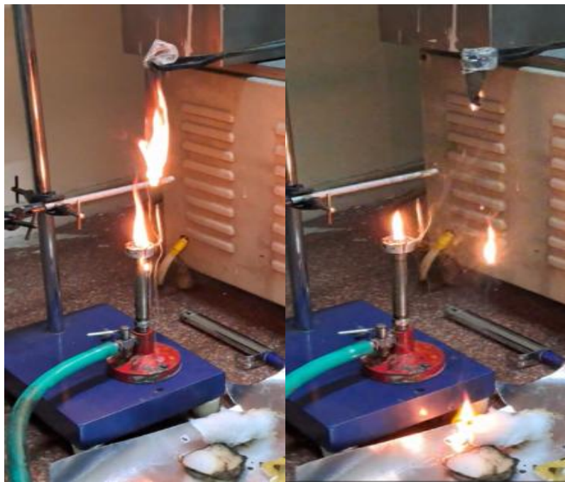
Fig.3.26: UL 94 vertical setup, and testing of the specimen
