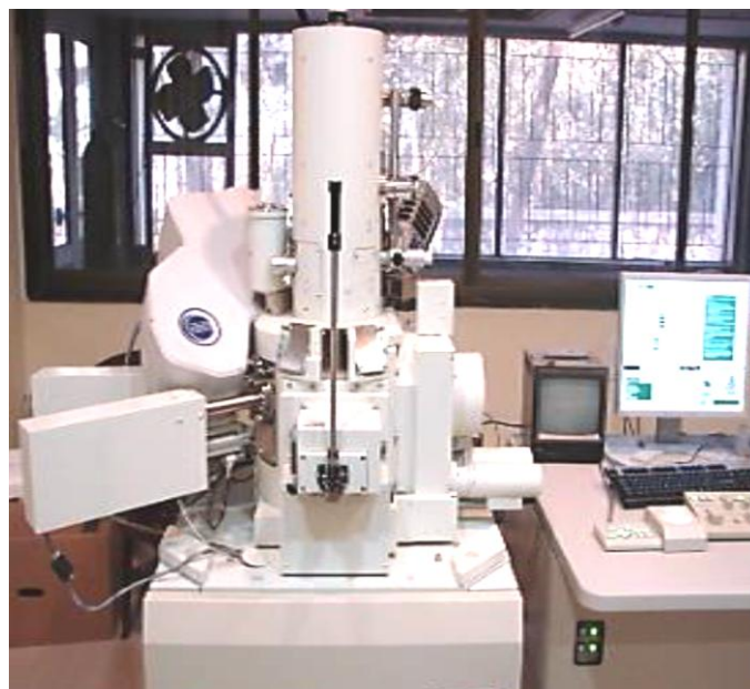
Fig. 3.8 Field emission gun (FEG) scanning electron microscope (SEM) for EBSD
