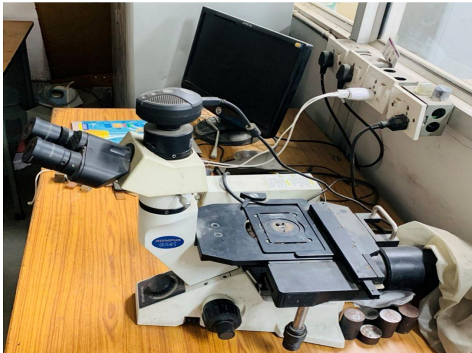
Fig. 3.7 Olympus GX41 compact inverted metallurgical microscope
