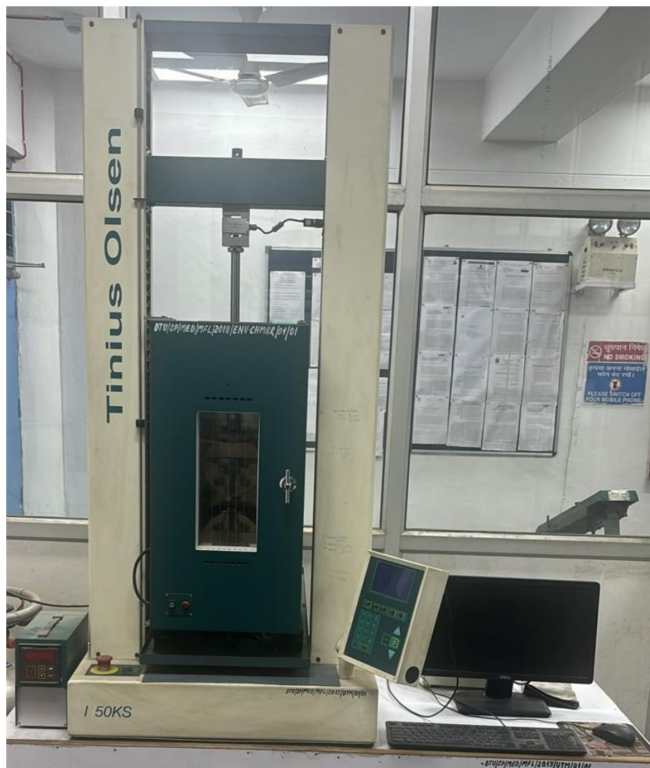
Fig. 3.3 Tensile machine (Model: Tinius Olsen H50KS)
