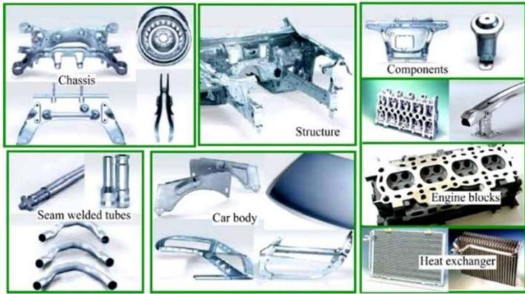
Figure 1.11 Applications of aluminum alloys in automobiles [45]
