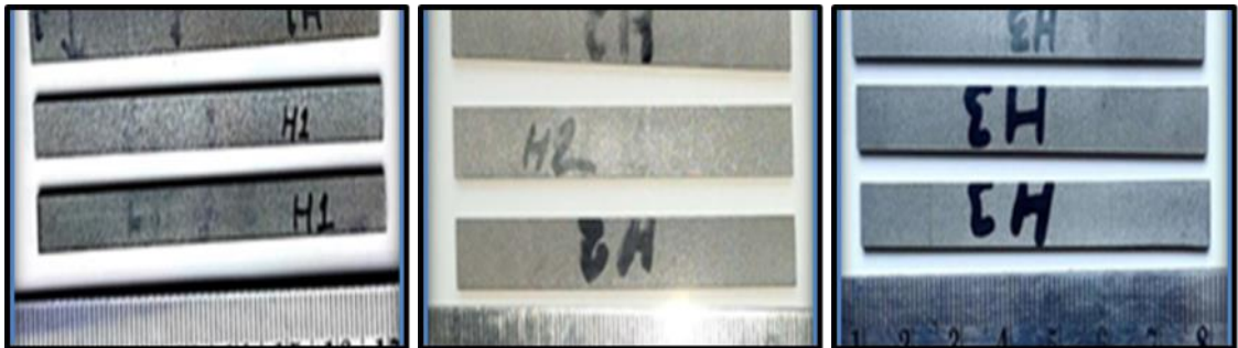
Figure 5.3: T6 Heat-treated test specimens for 8, 12, and 16 wt. % B 4 C
