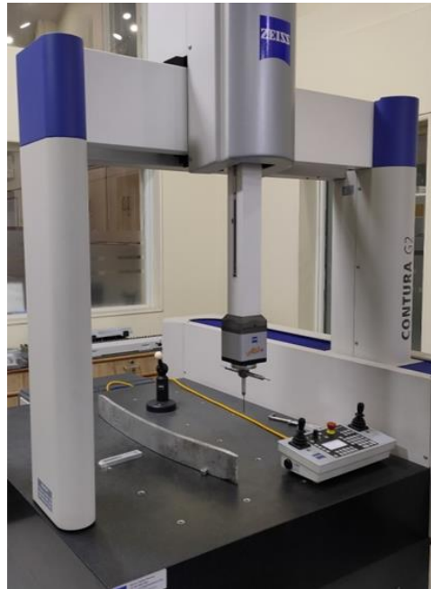
Figure 6.1: Measurement of leaf spring geometry using CMM.
