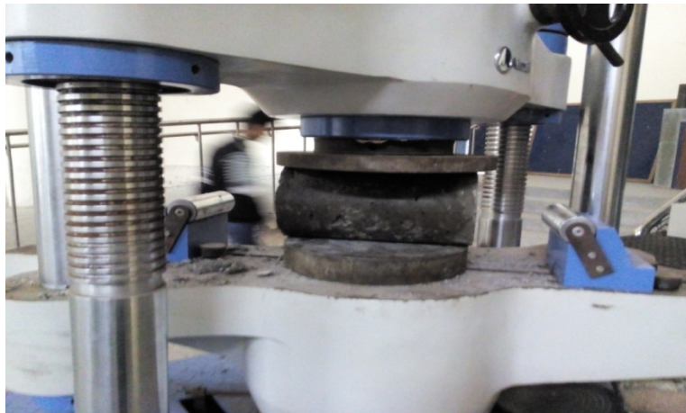
Figure 4.7 Arrangement for splitting tensile strength test
