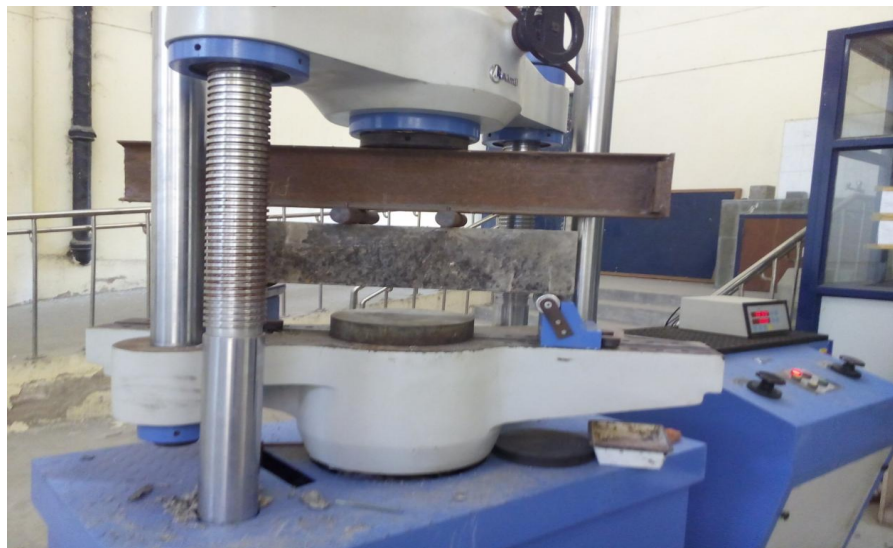
Figure 4.4 Arrangement for flexural strength test
