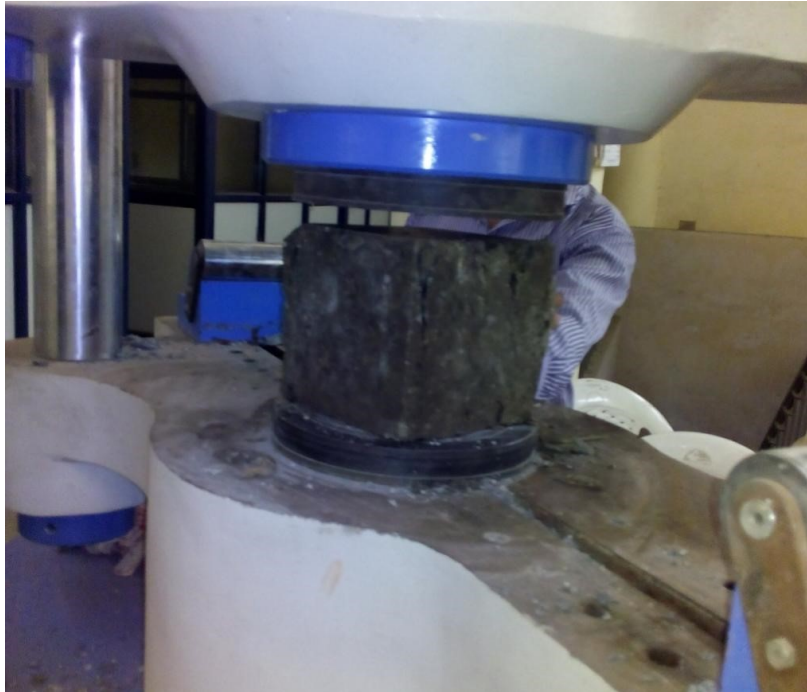
Figure 4.1 Arrangement for compressive strength test
