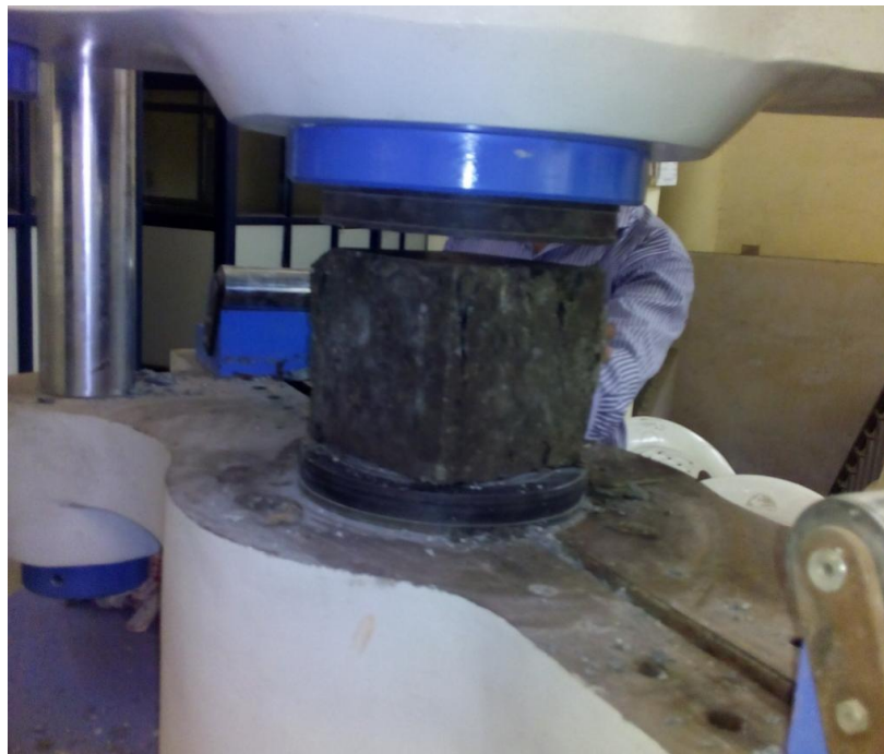
Fig. 4.1 Arrangement of a cube for compressive strength test
