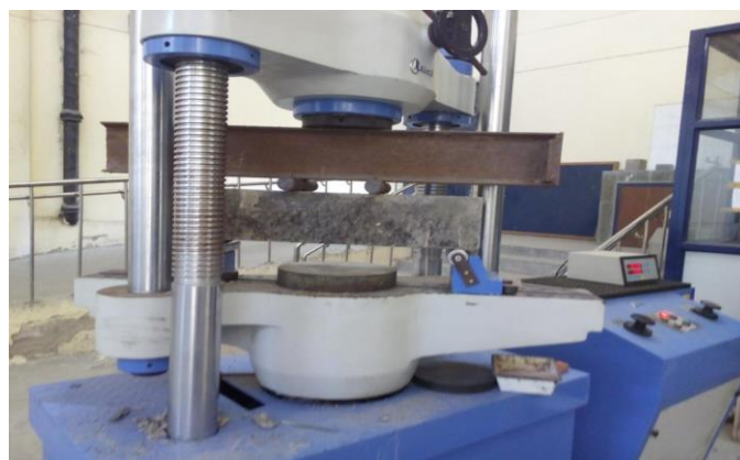
Fig. 4.4 Arrangement for flexural strength test
