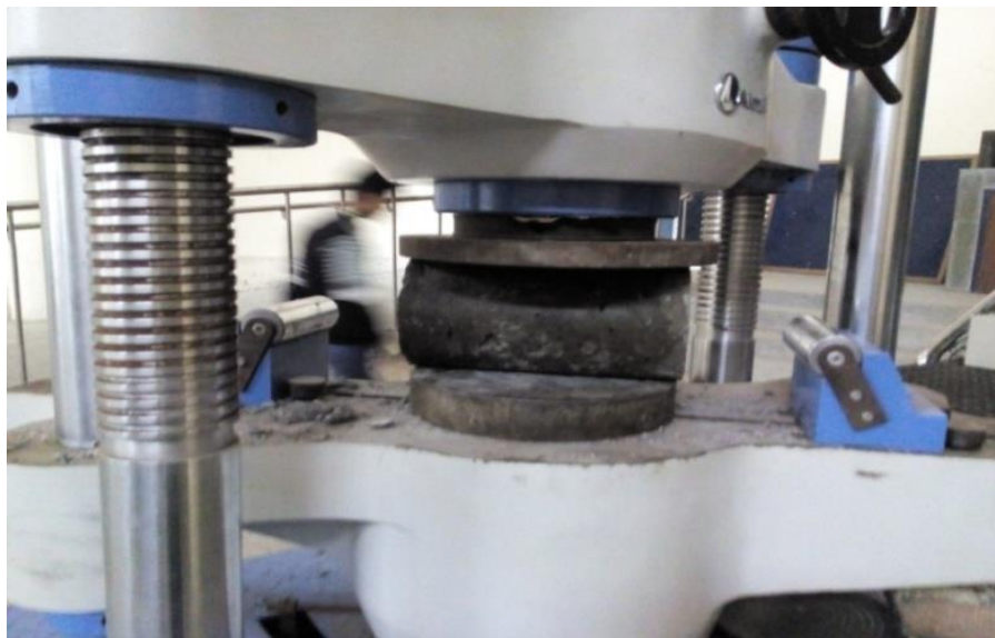
Fig. 4.7 Arrangement for splitting tensile strength test
