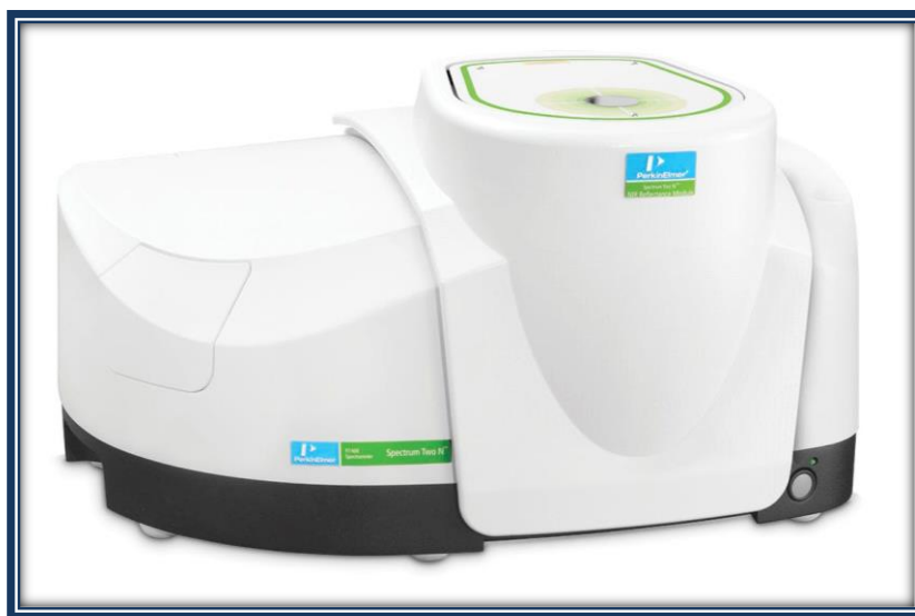
Figure: 2.4 spectrum two FT-IR spectrometers (Perkin Elmer)
