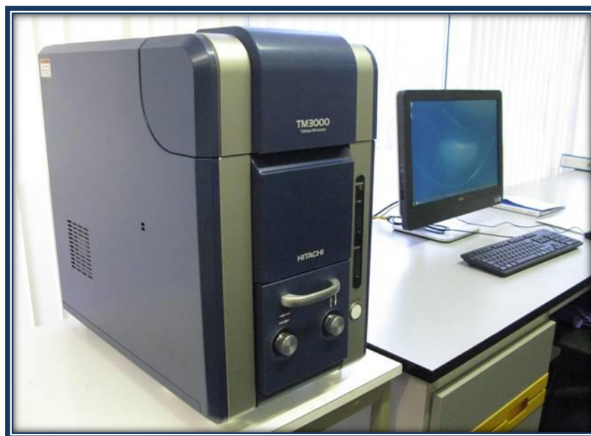
Figure:2.6 TM3000 Tabletop microscope.
