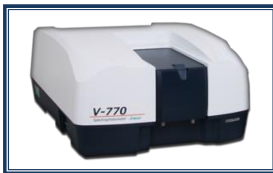
Figure:2.7 UV–vis spectrophotometer (Jasco V770).
