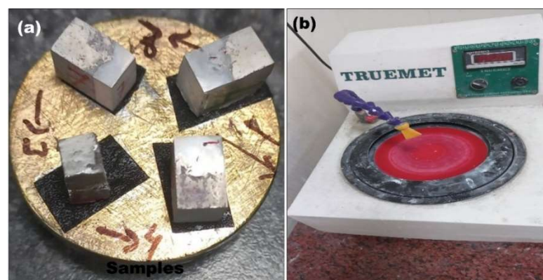
Figure 3.8:(a) Metallographic Samples (b) Single Disc Polisher
