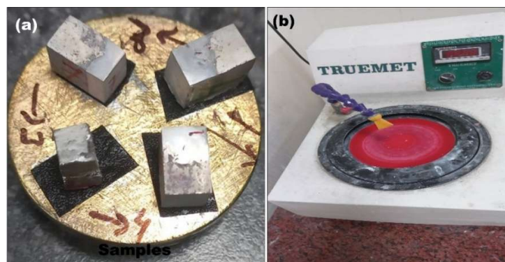
Figure 3.8:(a) Metallographic Samples (b) Single Disc Polisher
