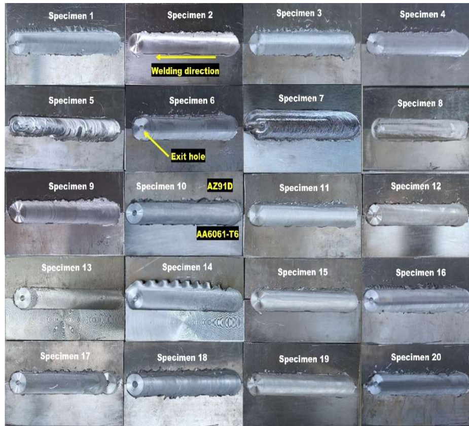
Figure 3.6: Top view of SiC reinforced FSWed samples of AA6061-T6 and AZ91D showing surface appearance
