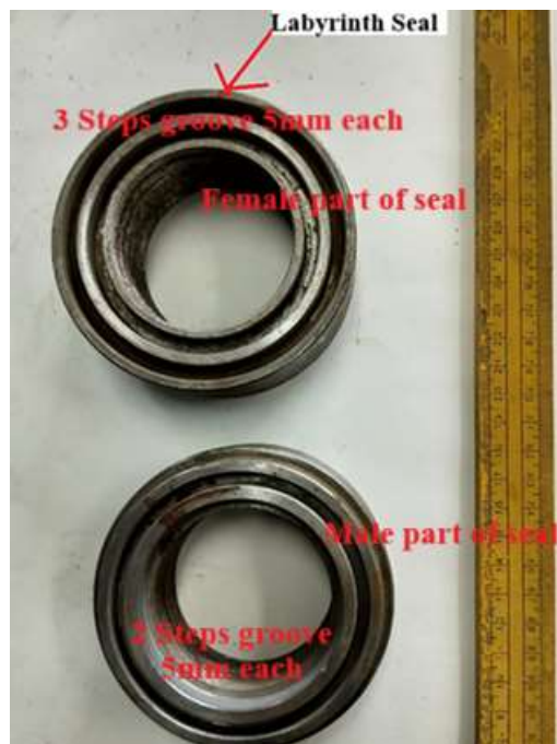
Fig. 3.12 Alloy steel EN24 metal Labyrinth seal
