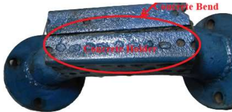
Fig. 1.6 Strengthening of pipe bend by concrete reinforcement [4]
