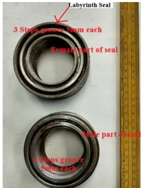
Fig. 3.12 Alloy steel EN24 metal Labyrinth seal
