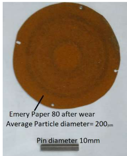
Fig. 4.1 POD wear impressions on emery 80
