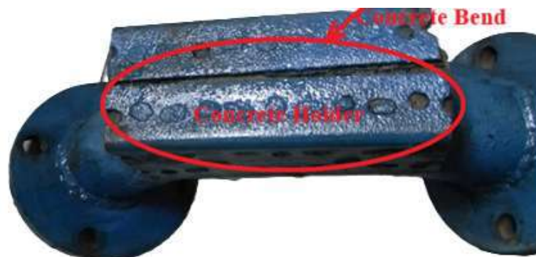
Fig. 1.6 Strengthening of pipe bend by concrete reinforcement [4]
