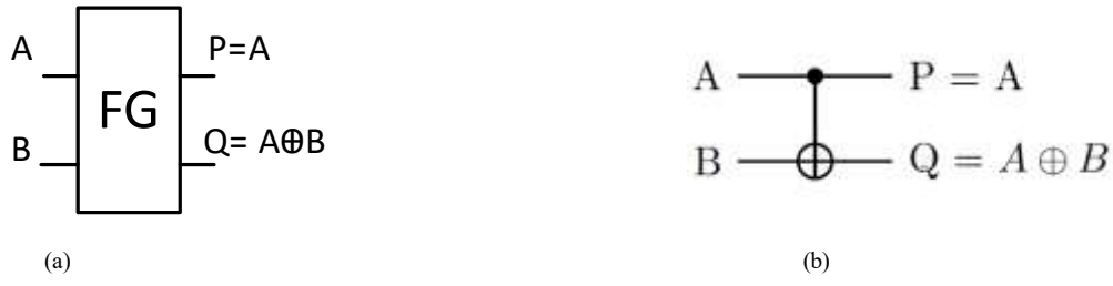
Figure 3.1: (a) Schematic depiction of the FG gate; (b) The quantum structure of the FG gate
