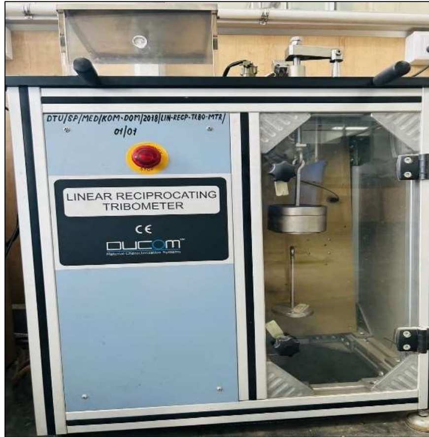
Fig. 4. 8 Linear Reciprocating tribometer (ASTM-G133)
