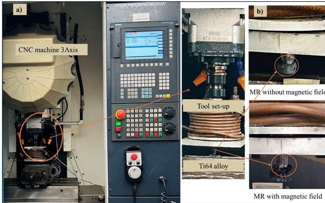
26 Fig. 4. 5 CNC machine with Setup tool (a), MR finishing under the effect of the magnetic field, and without the influence of the magnetic field (b)
