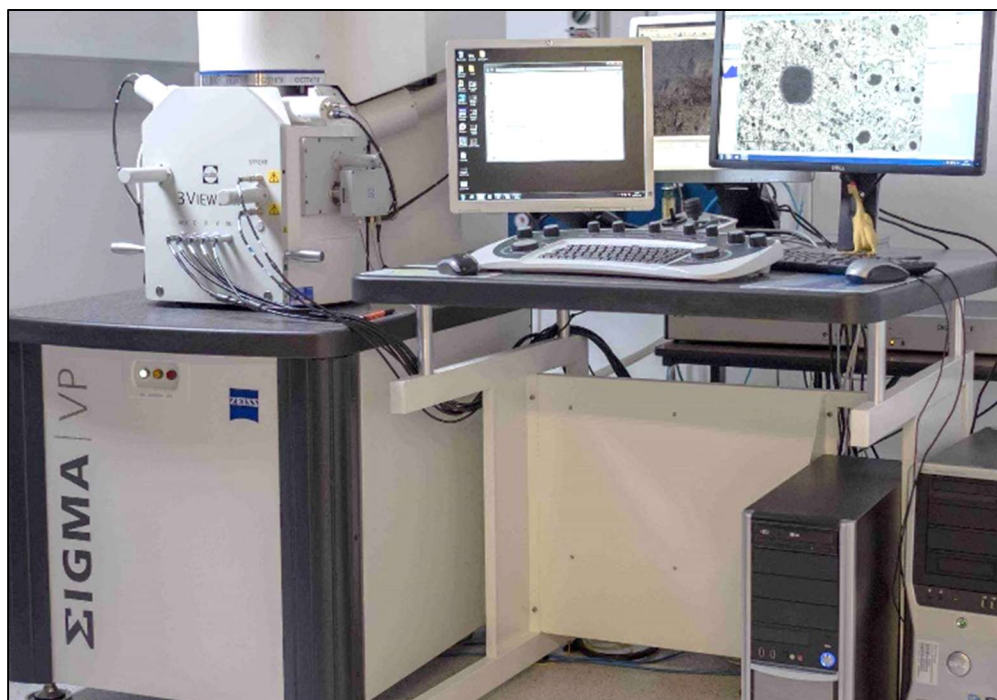
Fig. 4. 6 Scanning Electron Microscope attached with an EDS detector.
