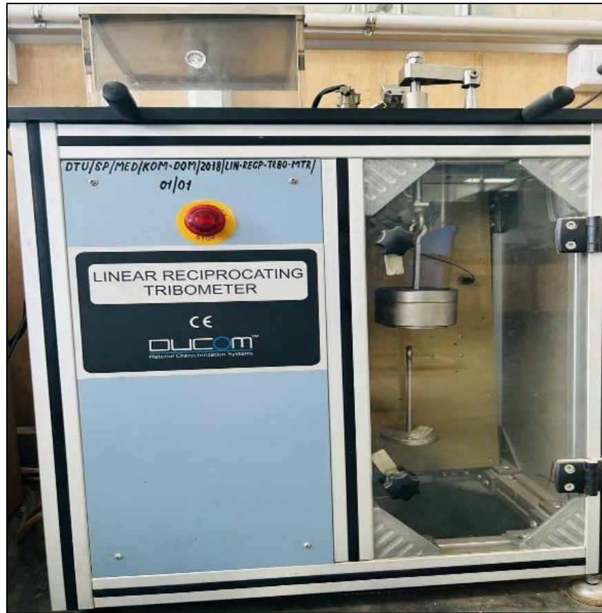
Fig. 4. 8 Linear Reciprocating tribometer (ASTM-G133)
