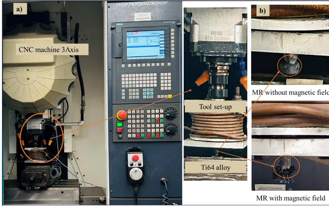
Fig. 4. 5 CNC machine with Setup tool (a), MR finishing under the effect of the magnetic field, and without the influence of the magnetic field (b)
